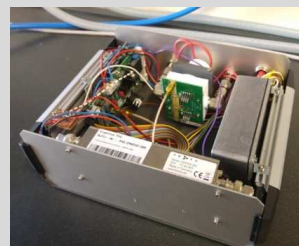
Fig. 2: Main components of our proof of principle gas analyser system with integrated FAIMS chip.
